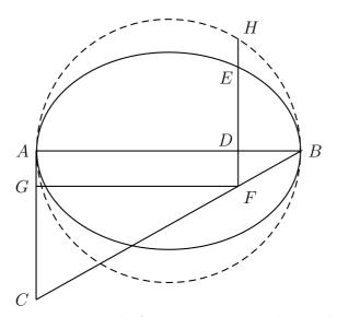
*Remark.* The ellipse appears to result from contracting the circle in one direction. If this is so, then by Newton's Lemma 4, the ratio of ellipse to circle is the factor of contraction, which should be DE/DH. So one should find this ratio and check that it is indeed independent of the choice of D.
